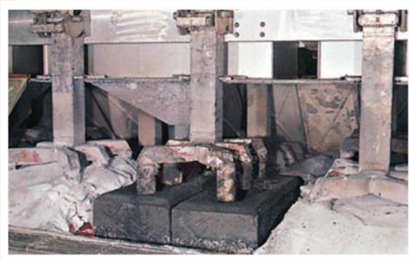
Horizontal prebaked carbon anodes in the HH cells.
