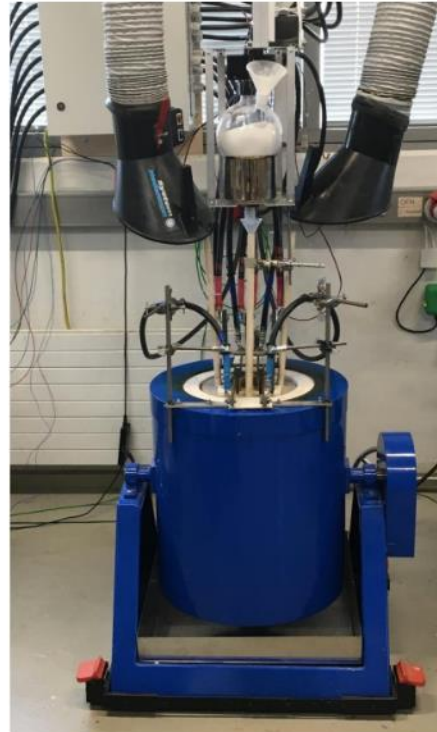
Electrolytic cell in electric furnace with power cables to the electrodes and alumina feeding device.
